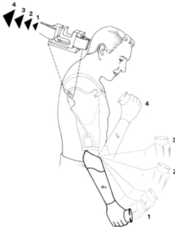
Fig. 3. Direct relationship of force to elbow positioning can be found in the Motion Control Servo Pro Force Sensor. (courtesy of Motion Control, Inc).
