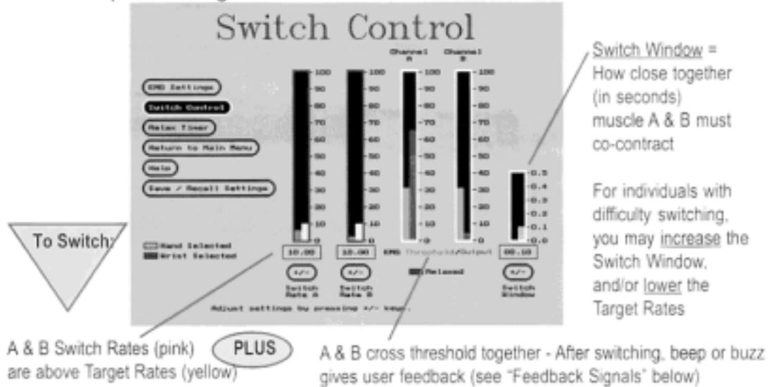
Fig. 11. Pro Control II Switch Control Window accessed for adjustment of co contraction switching between wrist and hand function. (courtesy of Motion Control, Inc).
