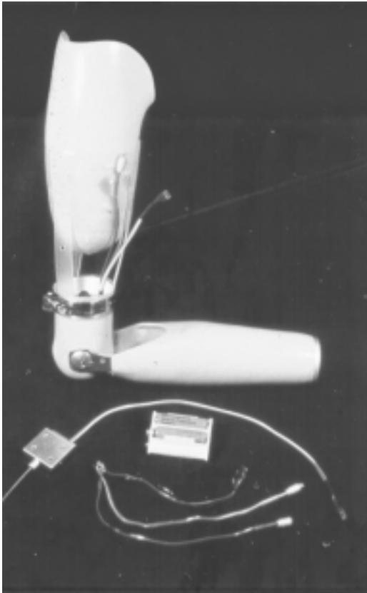
Fig. 1. Prosthesis Utilizing Switch Control.
