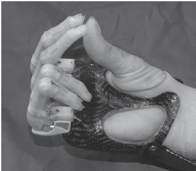
Figure 5. Use of the hypothenar compartment of the anatomical partial hand interface to promote sensation and stability.
