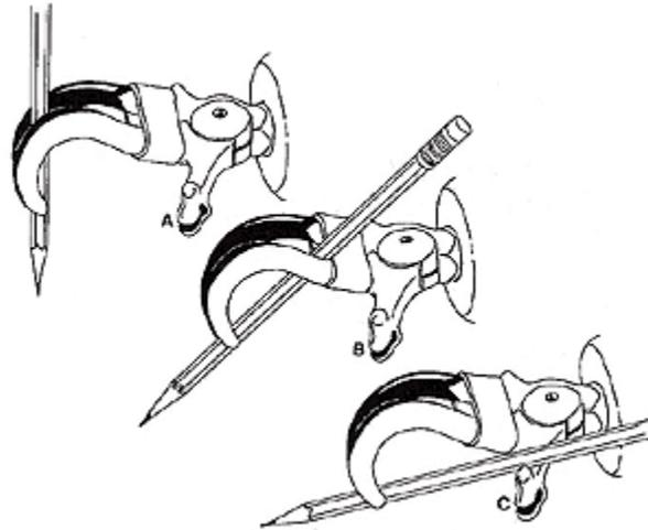
Figure 7. Holding a pencil with the terminal device is a difficult task. In "A" the pencil is not stabilized and is free to rotate in a clockwise direction. In "B" the pencil is stabilized against the tension band. In "C" the pencil is optimally stabilized against the thumb of the terminal device.
